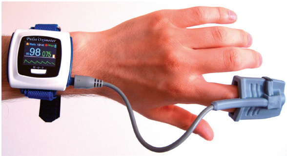
Fig. 17.2 A pulse oximeter attached to a finger continuously measures the level of oxygen in a patient's blood throughout an operation.
